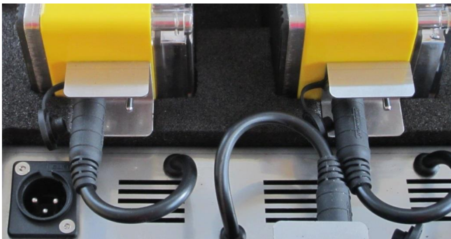
Lights correctly installed and connected in the case for charging
