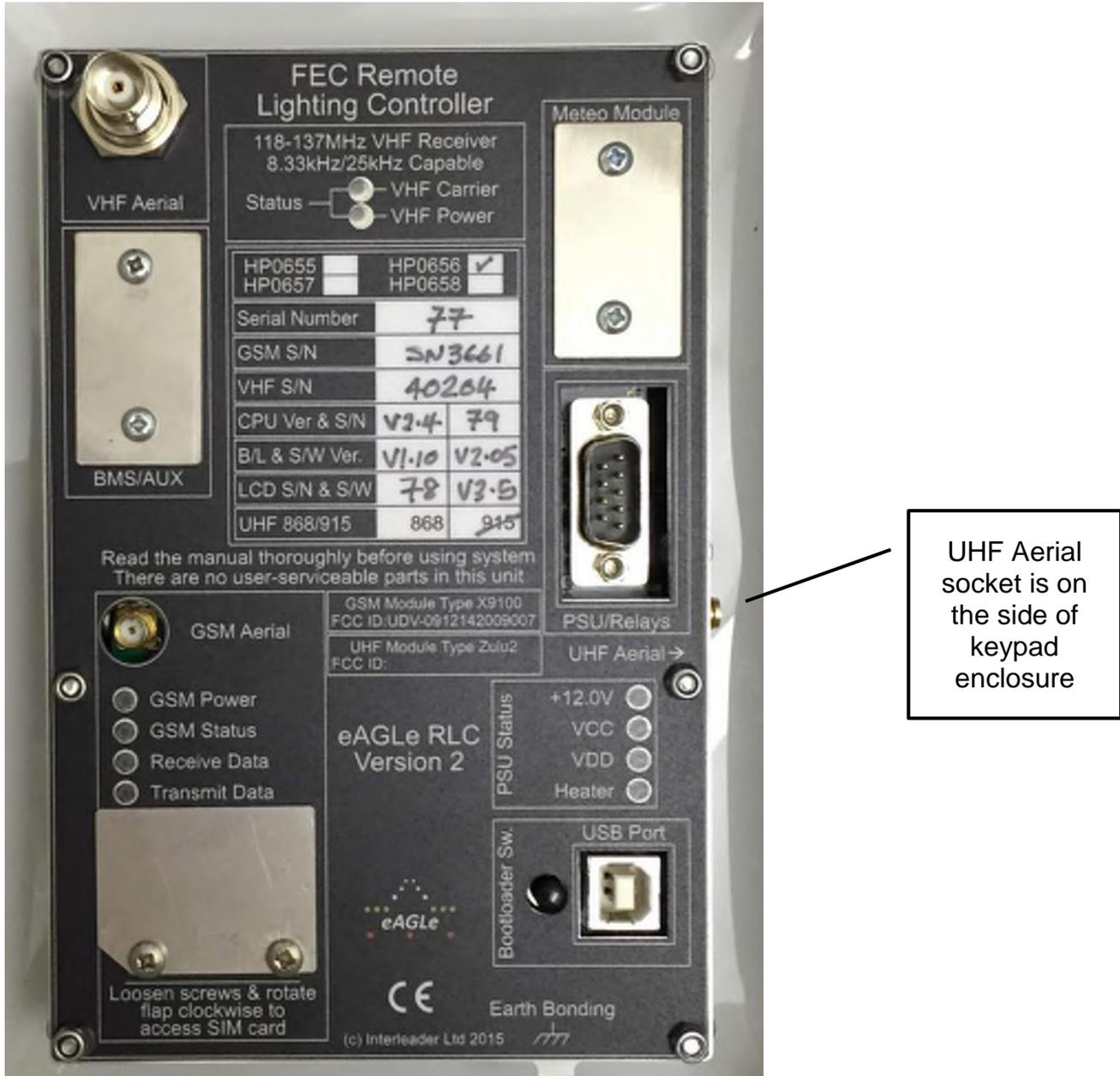
The UHF socket is on the side of the keypad enclosure where indicated. Care should be taken when removing and fitting the plug and it is best gently tightened with a slim jaw 8mm open-ended spanner.
