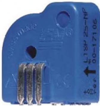
To achieve this the PSU and Relay interface Board has a non-contact current measuring transducer for each circuit (left). Each transducer is capable and calibrated to measure AC currents up to 20A and the software is designed to detect this circuit current.
