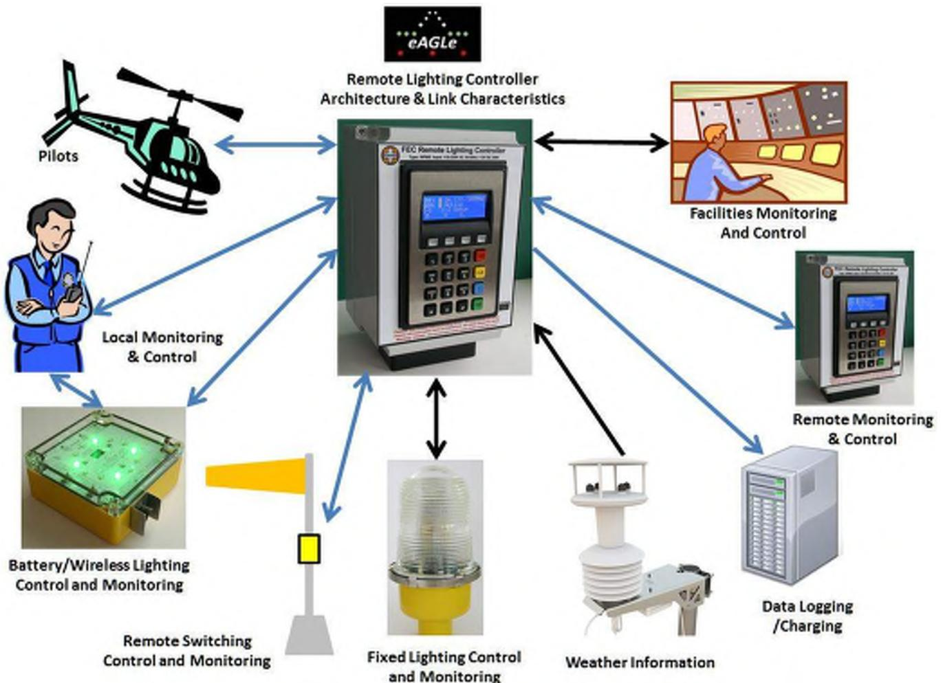
**NB – Battery/Wireless (868MHz UHF) UK/EU/ROW - (915MHz UHF) USA**
