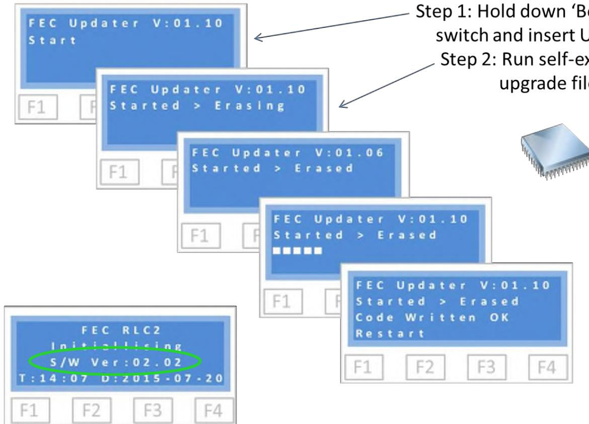
The first that the RLC is started after a software update pay attention to the initialisation screen and confirm version of software is as expected. Repeat with the correct version if not.
