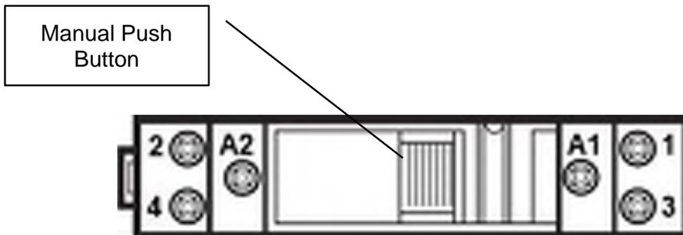
This will make the contact for the normally open contact and break the contact for the normally closed contact.
