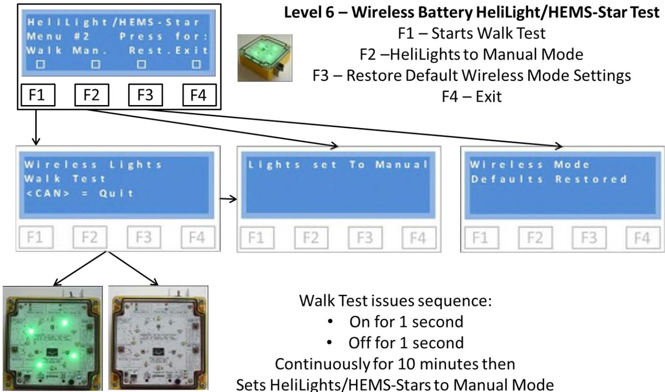
To perform a Walk Test, press F1 and the RLC will send alternating On and Off commands every second (1 second On, 1 second Off) and will continue to do for either:
