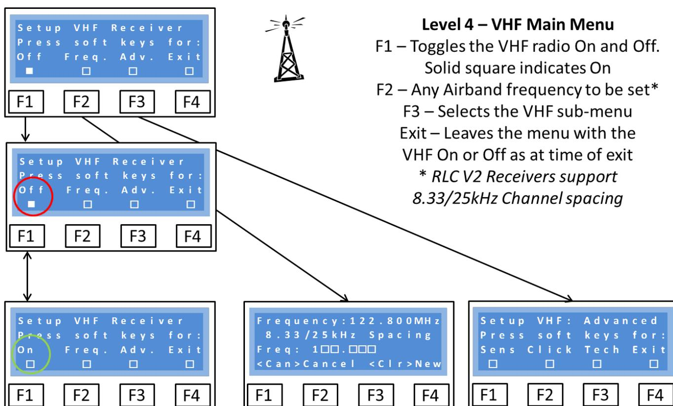
Note that the VHF radio is toggled On/Off using F1 and is set in that state when exiting the menu using F4. A solid square means 'On' and the action of the function key is to turn it off.
