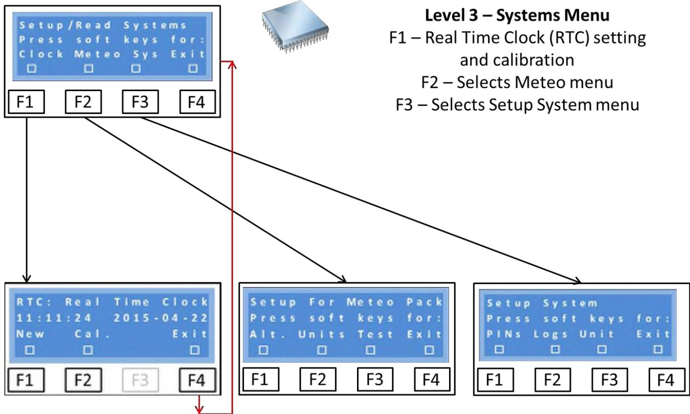
**Clocks** - The FEC RLC V2 has two, battery backed up, Real Time Clock/Calendars (RTC).
