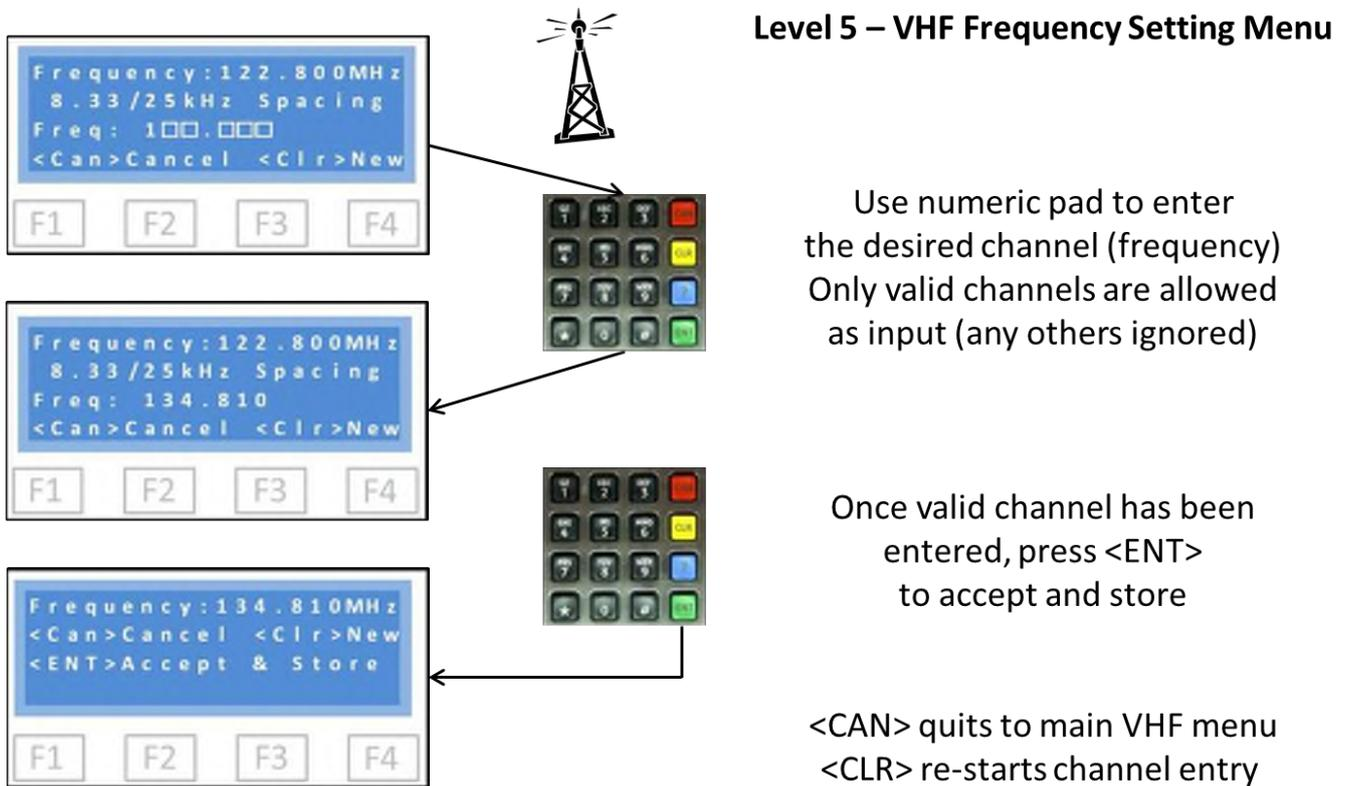
**Frequency (Channel) Setting** – as each number is entered it is checked to ensure that the frequency (channel) is valid. If valid the number entered is displayed and the cursor moves to the next space.
