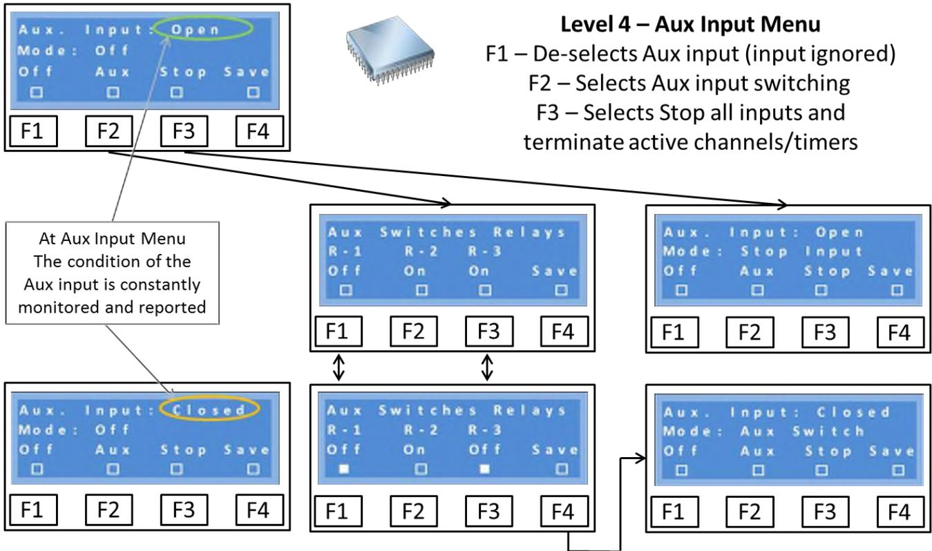
**Off Mode** - The default mode for the Aux input is Off. In this mode, whatever the status of the Aux input, it will be ignored.
