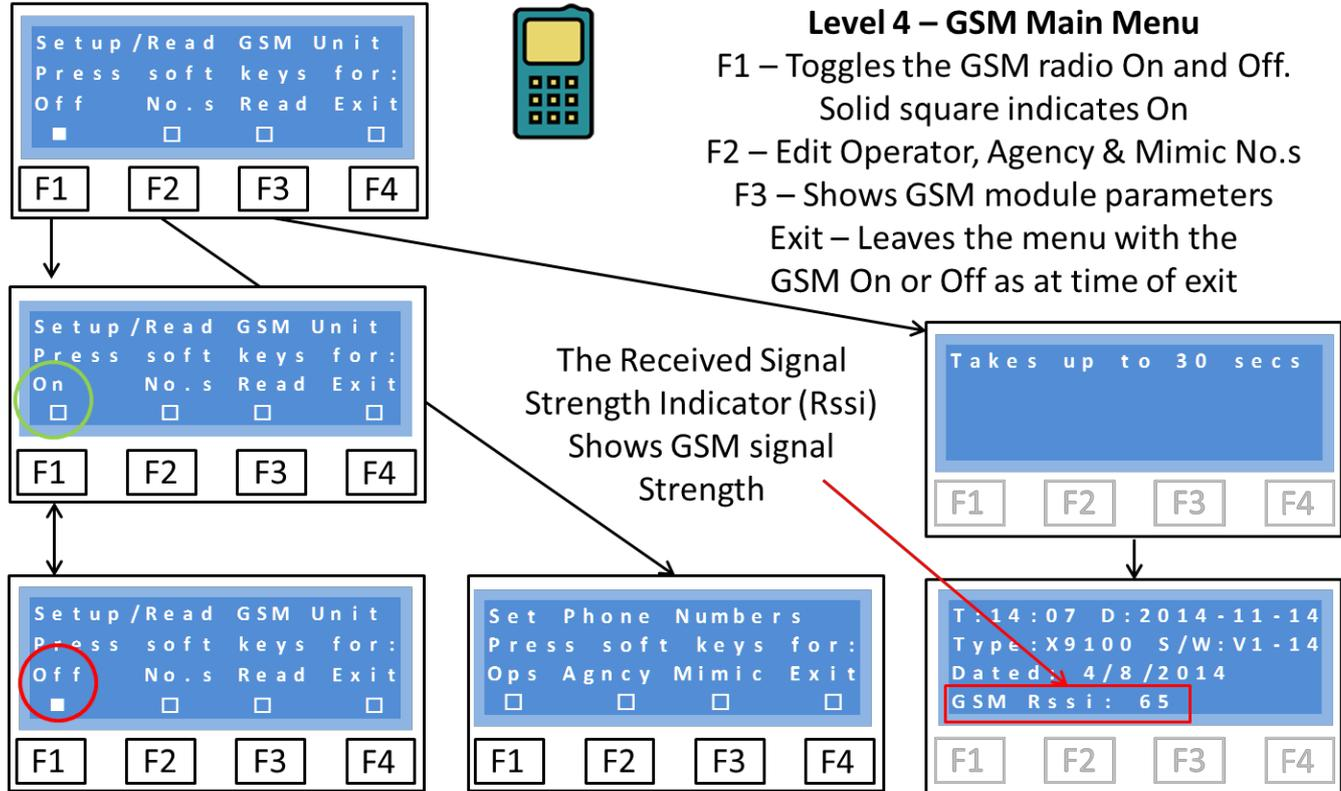
Note that the 1<sup>st</sup> soft key is solid indicating that the GSM receiver is ON and that the soft key option is to turn it Off. Pressing F1 will toggle the GSM receiver on and off and it will be left in that state on Exit. The other menu options are:
