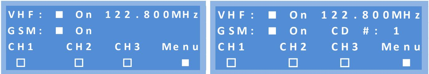
In this case Indicating that both VHF and GSM are ON but that no channel is active.
