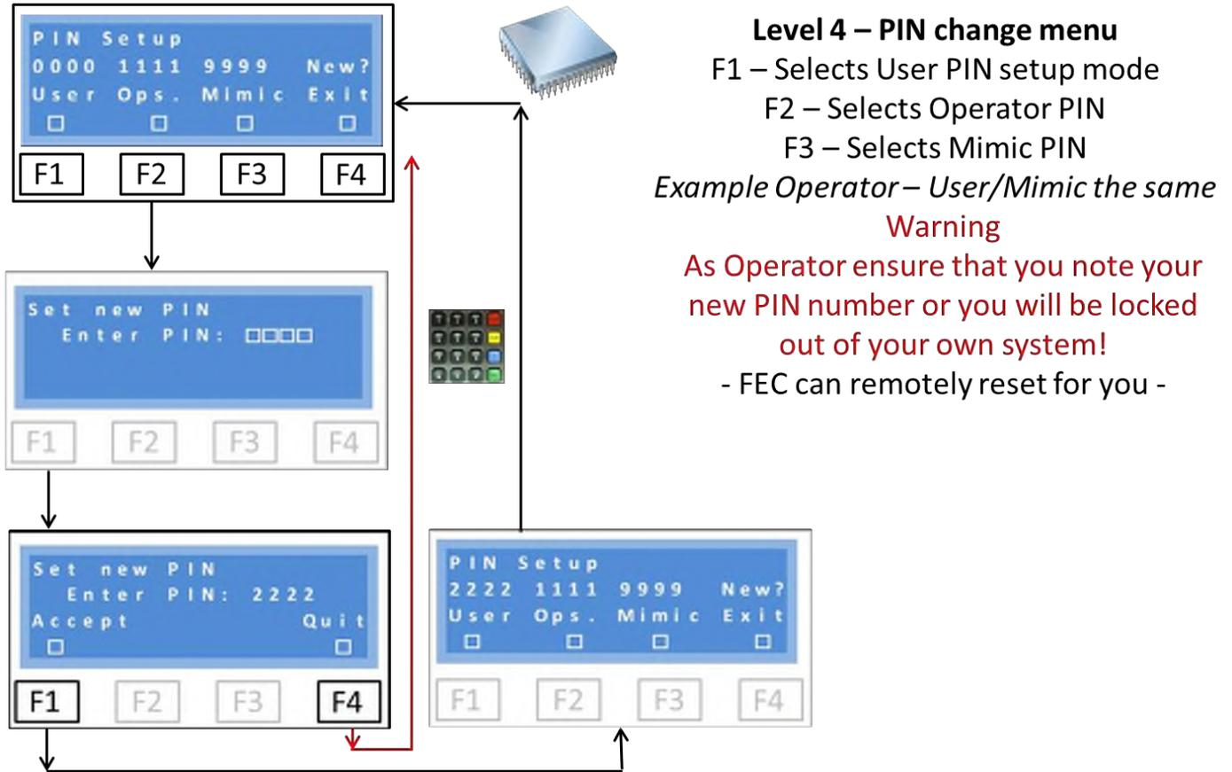
The above example shows how the Operator can reset their own PIN.
