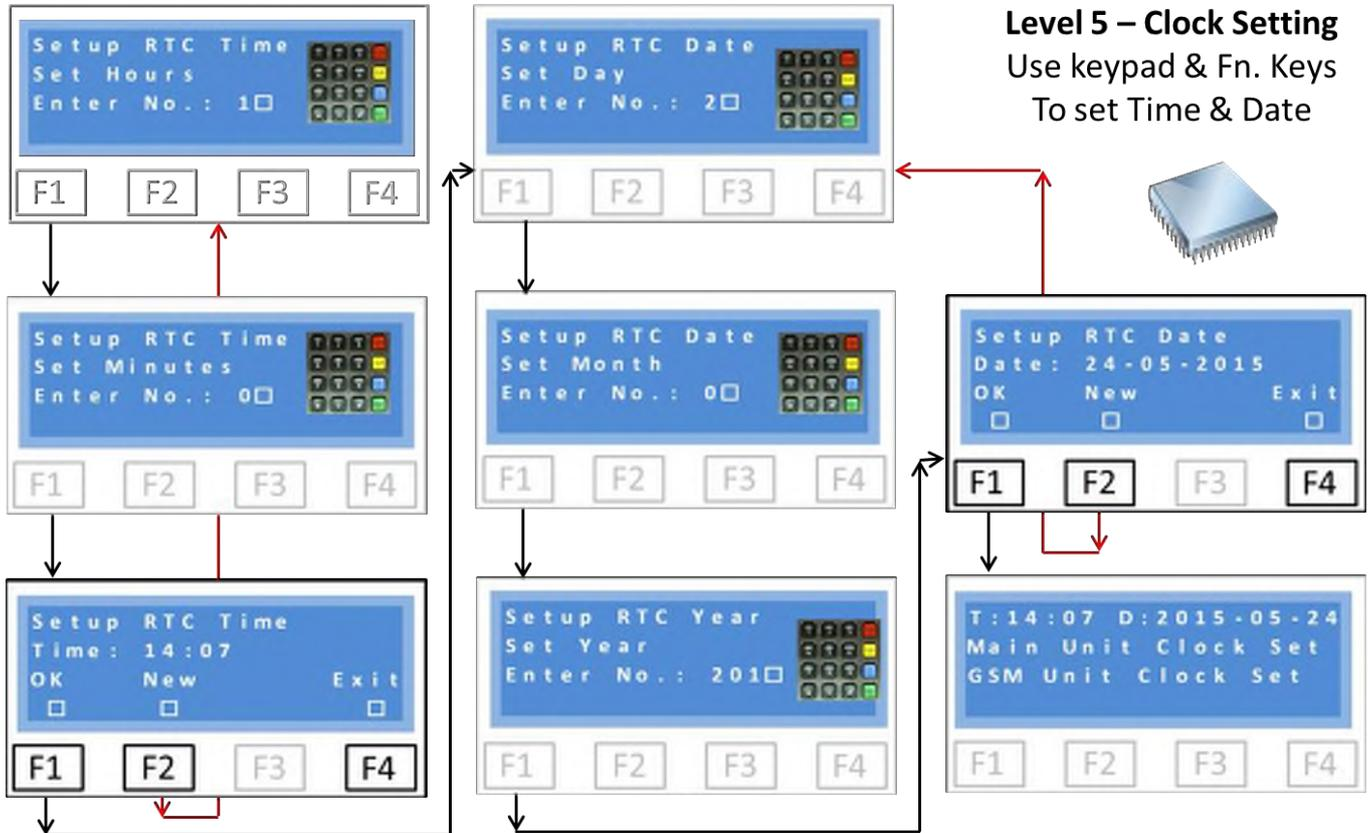
The first screen requests the hour. This must be entered in 24 hour format and as a two digit number. For example 9 o'clock in the morning would be entered '09' and 5 o'clock in the afternoon '17'.
