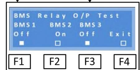
The Aux/BMS interface on the RLC supports 1 input and 3 outputs.
