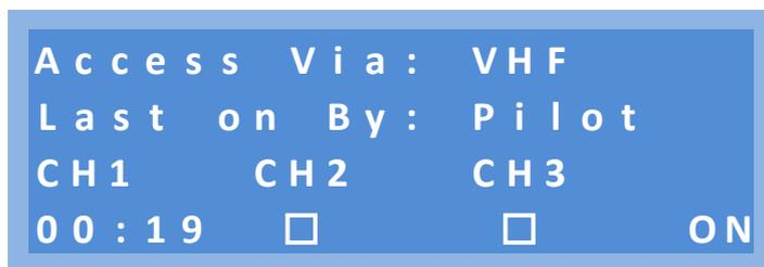
The above shows that Chanel 1 (Relay 1) is active (ON) and that the system is timing down. The time-out period is 0 minutes 19 seconds. At the end of this period the channel will be deactivated.
